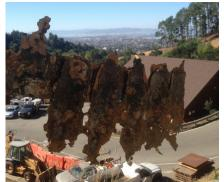
Corrosion in corrugated metal drainage pipes can often lead to structural deterioration and eventual collapse. Many owners are solving this problem by cement mortar lining drainage pipes before corrosion becomes detrimental. H&R Plumbing recently performed an application of Mainstay ML-72 Restoration Mortar on 50' of corrugated metal culvert using Madewell's horizontal mortar spinner.
