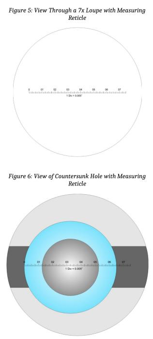
Coating film thickness is measured using a magnifier with a measuring reticle (Figure 5). In Figure 6, we are using a 7x loupe with a reticle capable of measuring <sup>3</sup>/<sub>4</sub> of an inch in .005" divisions (5 mils per hash mark). Note that when the measuring loupe is placed on top of the drilled hole, it is possible to measure the
