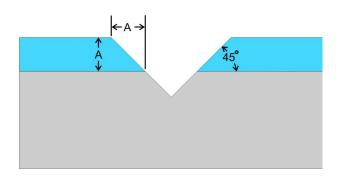
Figure 4: Counter Sunk Hole in Plan View
