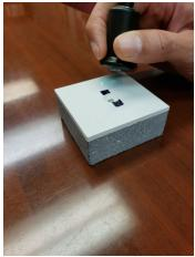
Photo 2: Ultrasonic Film Thickness Measurement
