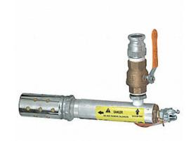
Bladder style vacuum testers can seal on the frame or at the top of the cone (images courtesy Cherne® Company).
